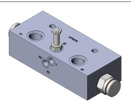
26 GPM, 3,000 PSI 6 PORT 2 POSITION SOLENOID CONTROLED PILOT OPERATED DIVERTER VALVE ASSEMBLY WITH #12 O-RING FUNCTION PORTS AND #6 O-RING PILOT PORTS. In the neutral position, no pilot pressure, oil will flow bi-directionally from the from A1 and B1 ports to the A2 and B2 ports with the A3 and B3 ports blocked. When piloted, oil will flow bi-directionally from the from A1 and B1 ports to the A3 and B3 ports with the A2 and B2 ports blocked.
