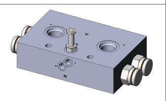
50 GPM, 3,000 PSI 6 PORT 2 POSITION SOLENOID CONTROLED PILOT OPERATED DIVERTER VALVE ASSEMBLY WITH #12 O-RING FUNCTION PORTS AND #6 O-RING PILOT PORTS. In the neutral position, no pilot pressure, oil will flow bi-directionally from the from A1 and B1 ports to the A2 and B2 ports with the A3 and B3 ports blocked. When piloted, oil will flow bi-directionally from the from A1 and B1 ports to the A3 and B3 ports with the A2 and B2 ports blocked.
